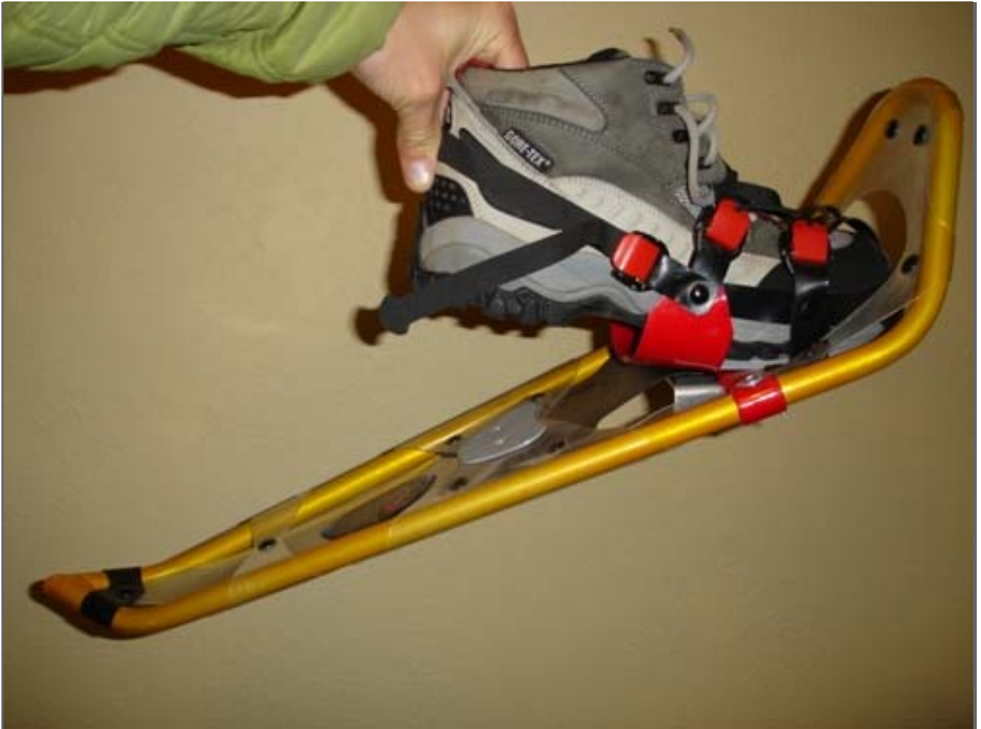
Crescent Moon uses a stiff pivot strap (red strap connected to the frame) to keep the snowshoes from dragging the ground.
